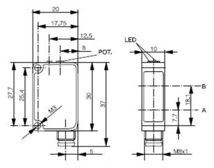
A: emitter axis B: receiver axis
