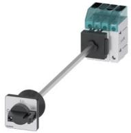
Load disconnector 3LD3, Iu 32 A Main switch 3-pole + N Rated operating capacity for AC-23 A at 400V 11.5kW floor mounting Basic switch with door coupling Central hole mounting 22.5mm Toggle drive black 48x48 mm
