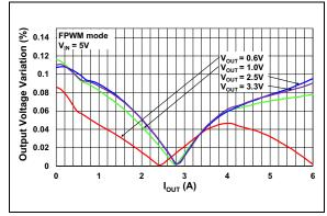
**FIGURE 2-11:** Load Regulation: V<sub>OUT</sub> Voltage Variation vs. I<sub>OUT</sub>.
