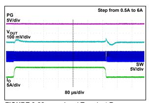
FIGURE 2-28: Load Transient Response.
