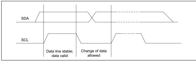
FIGURE 6-1: Bit Transfer Diagram.
