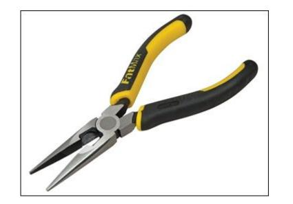
The Stanley FatMax Long Nose Pliers are made from heat treated high chrome steel forging for long life and durability. With a hand ground, induction hardened blade for long life and accuracy. Interlocking joint assembly for smooth cutting. Fitted with bi-material handles with secure grip grooving. Ideal for maximising grip and manoeuvring of small objects in confined spaces.
