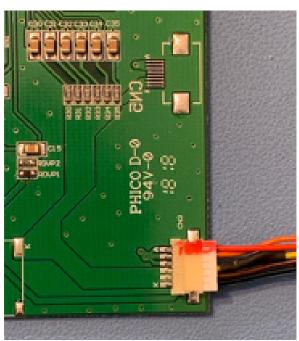
Observe the connector on the back of the display. Note that the connection pins are to one side of the black housing. Observe the connector on the end of the cable and note that the sockets are also at one side of the housing. The connector should be placed with the pins and sockets on the same side. If it is difficult to insert then it may be the wrong way round. Note that the manufacturer supplies two versions of this cable with opposite colours, so either may be inside your kit.
