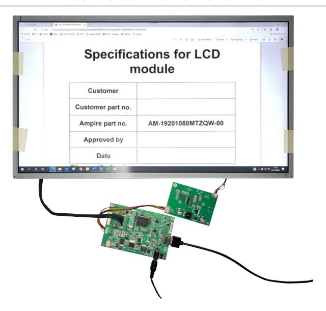
The connections are very fragile and easily torn. It is recommended that all connections are taped and all loose parts are insulated and taped to the rear of the display once the connections have been completed.
