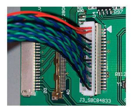
Connect the LVDS cable into the back of the display.
