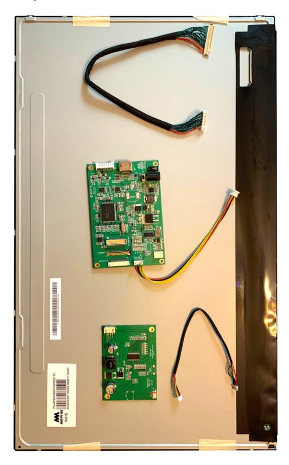
Locate the red mark on one end of the backlight connector.
