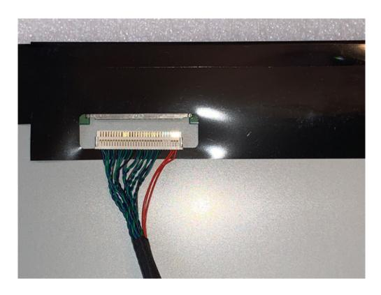
Align the connector with the contacts facing up as per the photo below.
