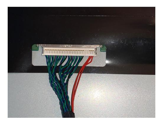
The connections should look like this when the connectors are connected correctly.
