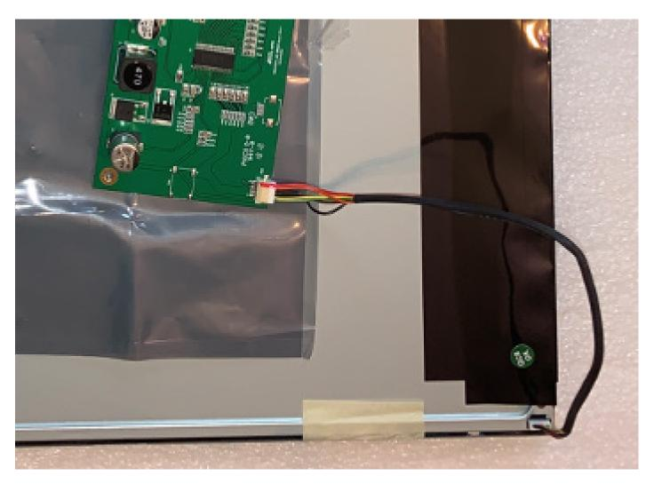
Connect the backlight power connection from the LVDS driver board.
