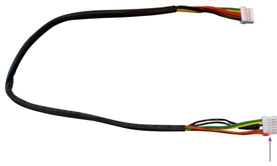
Connect the backlight cable into the backlight PCB
