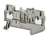
Terminal block, Linergy TR, grey, 2.5mm², push-in type, knife disconnect, 2 points, set of 50
