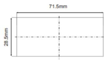
\*Panel thickness should be maximum 7mm.
