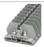
Bolt connection terminal block, Connection method: Bolt connection, Cross section: 2.5 mm² - 35 mm², AWG: 12 - 2, Width: 17 mm, Height: 39.7 mm, Color: gray, Mounting type: ct screw connection
