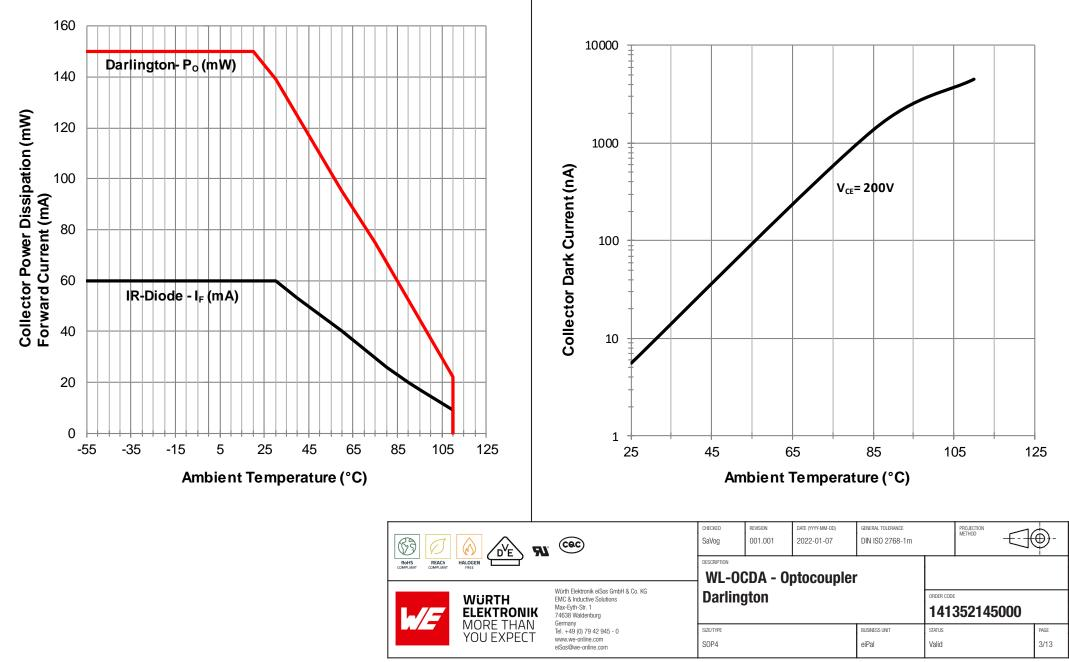
Collector Dark Current vs. Ambient Temperature:
