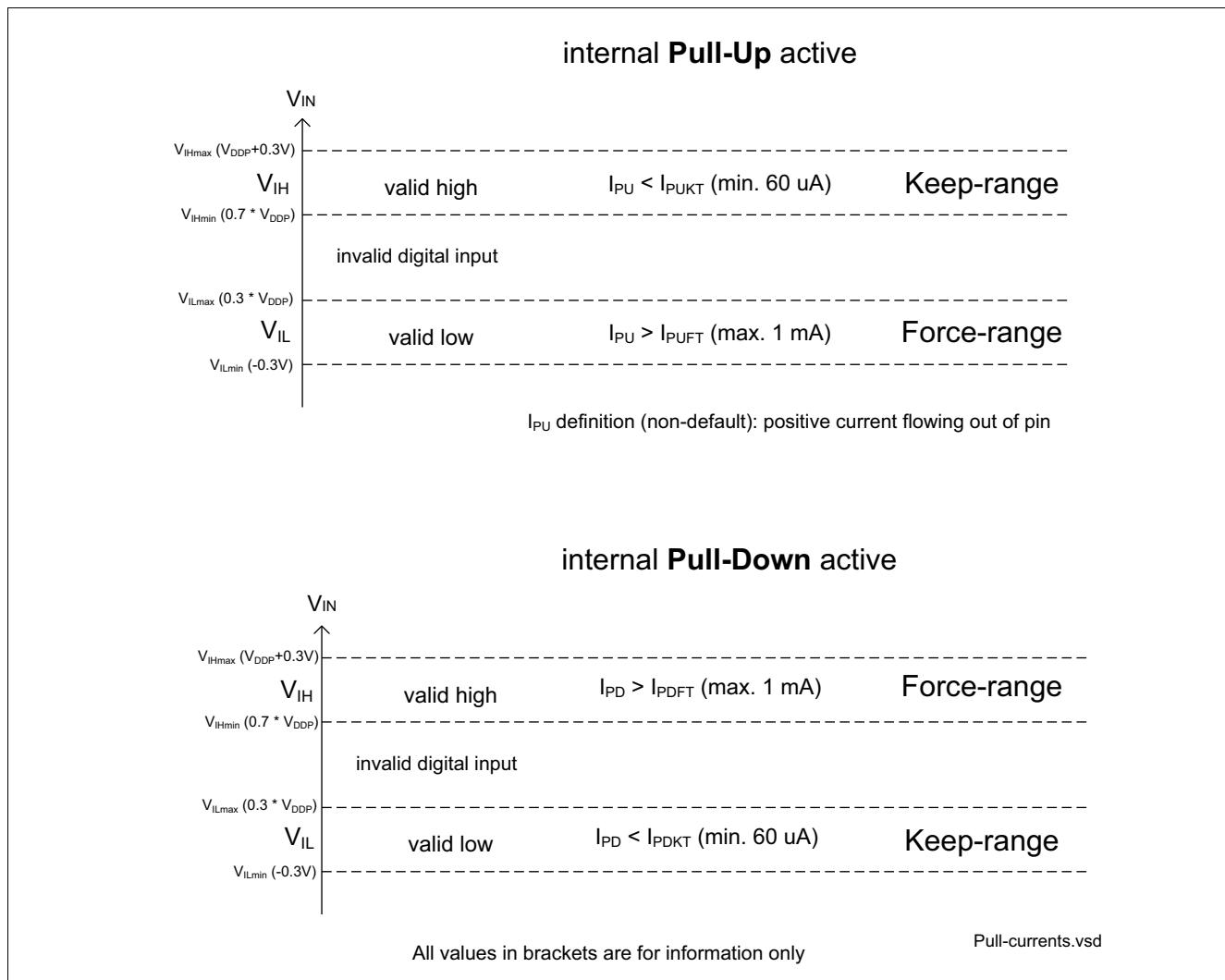
**Figure 23 Pull currents, Keep and Force Current**
