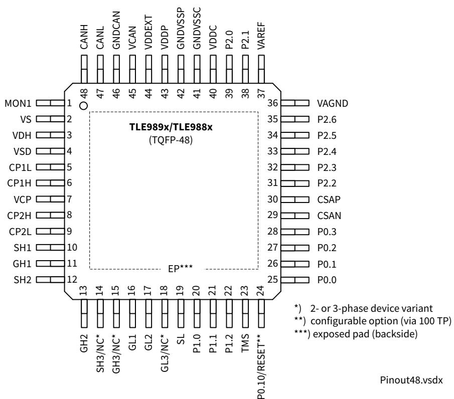
**Figure 2 Pinout for 48 pin package**
