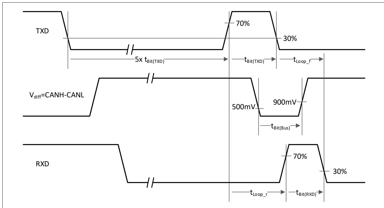
**Figure 19 From ISO 11898-2:  $t_{\text{loop}}$ ,  $t_{\text{bit(TXD)}}$ ,  $t_{\text{bit(Bus)}}$ ,  $t_{\text{bit(RXD)}}$  definitions**
