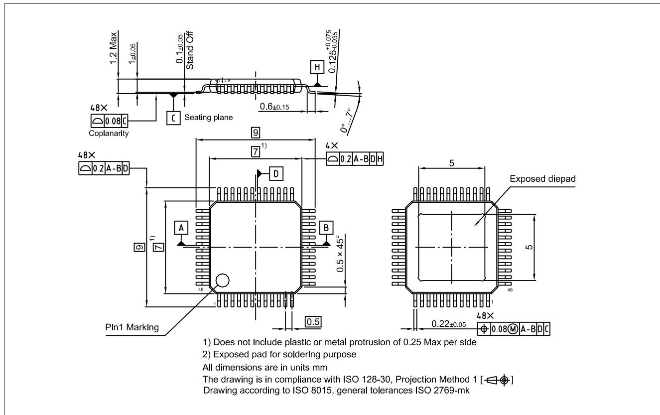
**Figure 46 PG-TQFP-48-10**
