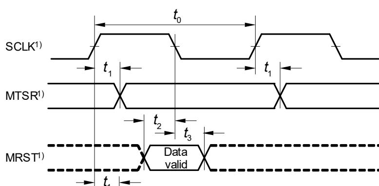
1) This timing is based on the following setup: CON.PH = CON.PO = 0.
