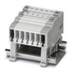
COMBI receptacle, Connection method: Push-in connection, Number of connections: 1, Number of positions: 4, Cross section: 0.14 mm<sup>2</sup> - 1.5 mm<sup>2</sup>, AWG: 26 - 14, Width: 14 mm, Height: 27.1 mm, Color: gray
