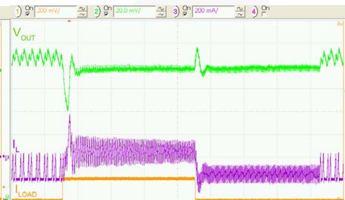
Figure 25. Load Transient 50 to 250mA, 2.5V_{IN}
