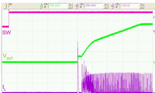
Figure 38. Soft-Start, R_{LOAD} = 50\Omega , 20\mu s/div.
