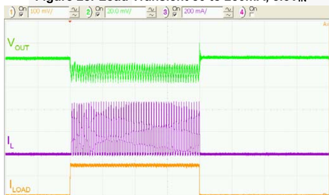
Figure 30. Load Transient 0 to 150mA, 4.5V_{IN}
