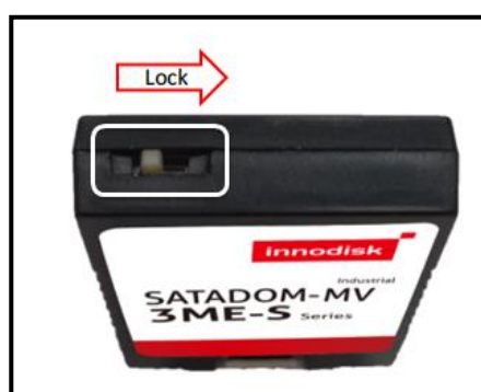
Figure 4: SATADOM-MV 3IE hardware write protect
