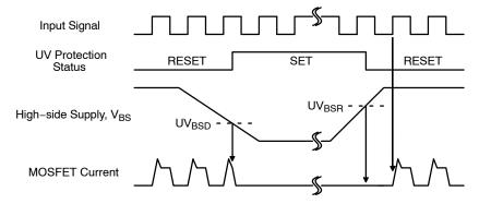
Figure 9. Under-Voltage Protection (High-Side)
