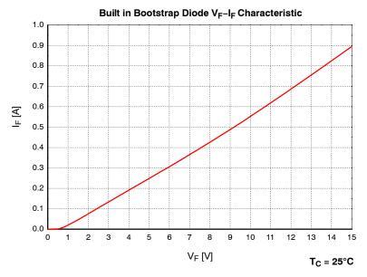
Figure 2. Built in Bootstrap Diode Characteristics (Typical)
