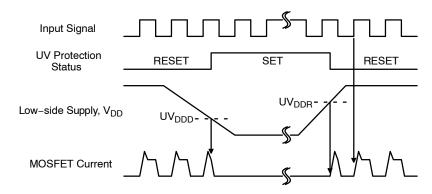
Figure 8. Under-Voltage Protection (Low-Side)
