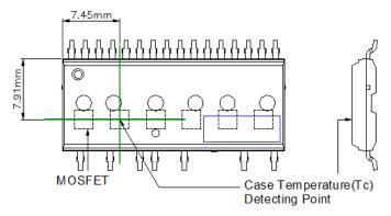
13. Attach the thermocouple on top of the heat-sink of SPM 5 package (between SPM 5 package and heatsink if applied) to get the correct temperature measurement.
