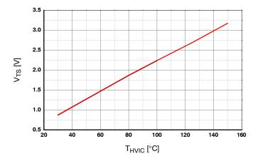
Figure 5. Temperature Profile of V<sub>TS</sub> (Typical)
