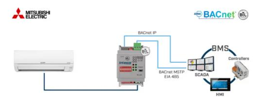
\*BACriet IP or BACriet MSTP communication selectable from switch configuration
