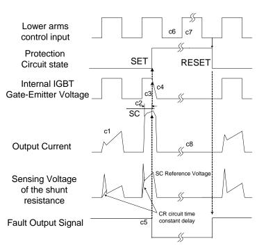
(with the external shunt resistance and CR connection)
