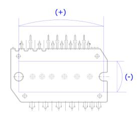
Figure 7. Flatness Measurement Position
