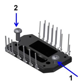
**Figure 8. Mounting Screws Torque Order**
