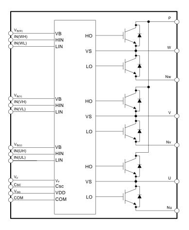
Figure 3. Internal Block Diagram
