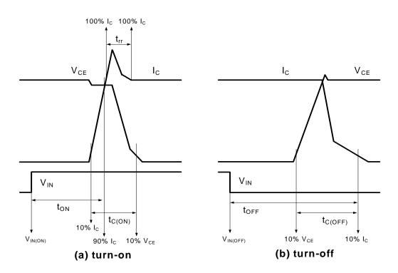
Figure 4. Switching Time Definition
