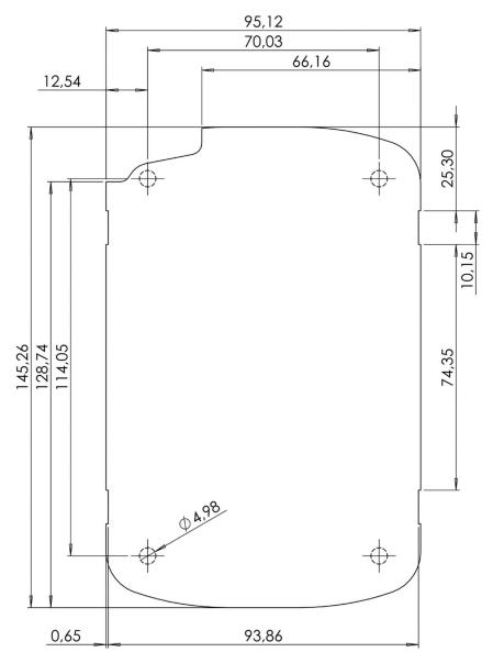
Dashed line shows outline of the mounting elements under PCB board Recommended mounting holes  $\varnothing 2,7$  All dimensions are given within +/-0,25mm tolerance
