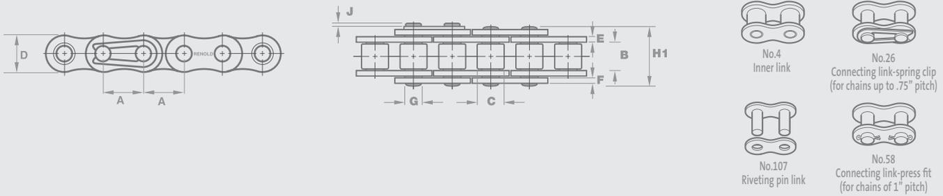
Renold standard power transmission chain can be adapted for conveying duties by the fitment of attachments shown on these pages. The attachments can be assembled on one or both sides of the chain at any desired pitch spacing.
