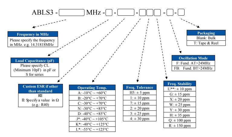
NOTE: Fundamental BT frequency stability ± 100ppm max. at -10° C to +60° C only.
