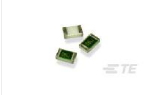
TE Part #8-1879214-9 CPF 0402 3K09 0.1% 25PPM 1K RL
