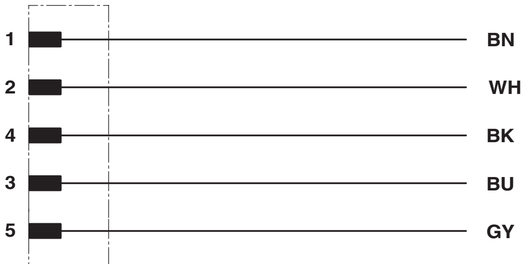
Contact assignment of the M12 connector
