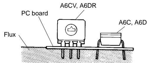
Both hand and automatic soldering are possible, under the following conditions:
