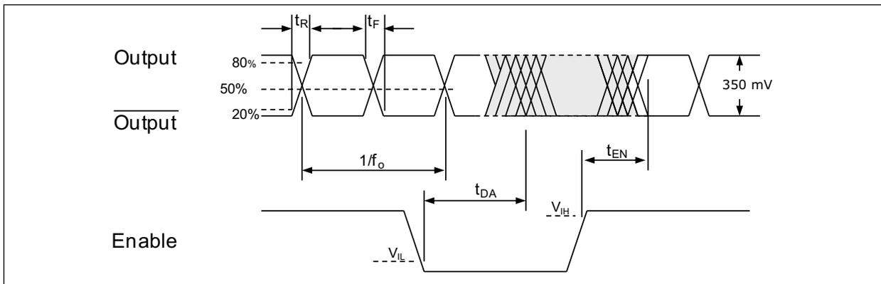
**FIGURE 3-3:** Output Waveform.
