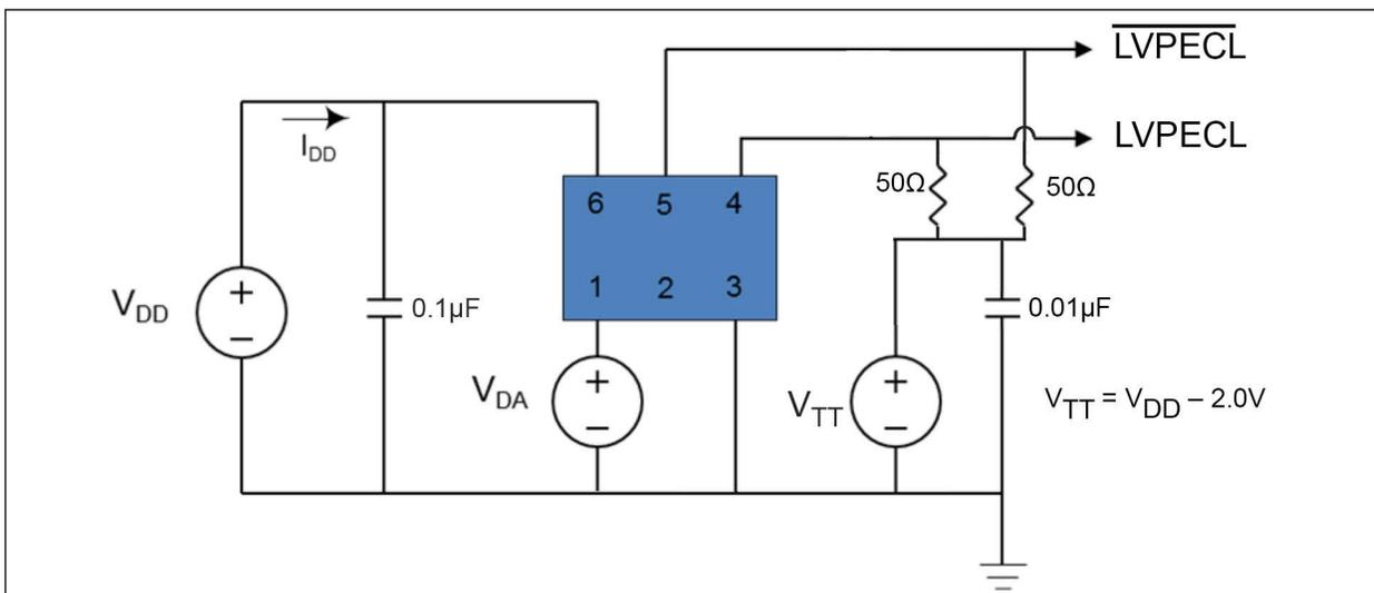
**FIGURE 3-5:** Test Circuit.
