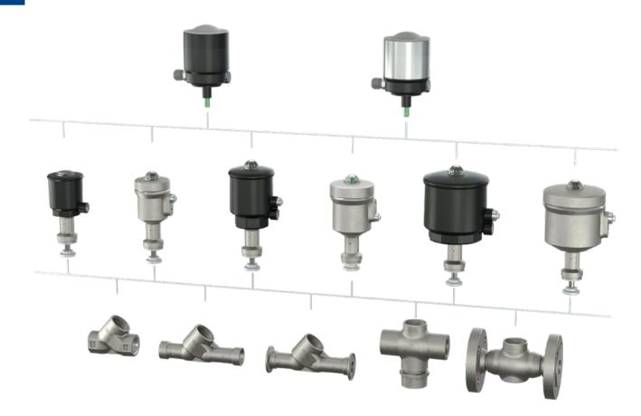
The modularity of the ASCO Series 290 makes it possible to interchange actuators of different size and materials on the same body. This allows quick and easy modification of the valve characteristics after assembly on site. This is very useful when mounting valves on a manifold block. Any combination of the broad range of different sized actuators, bodies and various switchbox types can be used.
