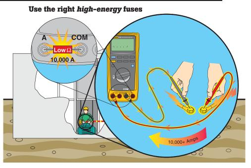
Figure 3. Misuse of DMM in Ammeter Mode.
