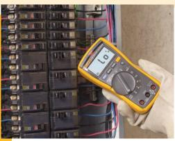
This meter has a built-in non-contact voltage tester.
