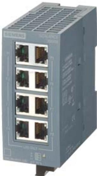
SCALANCE XB008 UNMANAGED INDUSTRIAL ETHERNET SWITCH POUR 10/100MBIT/S; AVEC 8 X 10/100MBIT/S TWISTED PAIR- PORTS AVEC PRISES RJ45; POUR LA CONST. DE PETITES STRUCT. EN ETOILE ET EN LIGNE; DIAGNOSTIC LED, IP20, ALIM. EN TENSION 24 V CC, AVEC MANUEL
