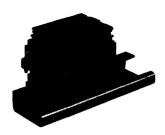
This accessory permits the interconnection of consecutive or non-consecutive blocks. For this, detach the studs manually where connection is not required. The use of two bars permits alternated jumping.
