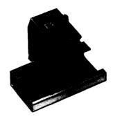
This accessory is for connecting or disconnecting two consecutive blocks, open or closed. The use of a third non-connected block is recommended, to allow for a "rest" position of the rotating jumper link. We recommend the use of a circuit separator in order to preserve the insulation. The BJP is mounted in the center of the terminal blocks, the connector bars of which are tapped for receiving the interconnection accessories.
