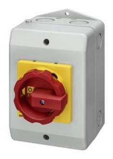
EMERG. STOP SWITCH 3-POLE IU=32, P/AC-23A AT 400V=11.5KW 1NO+1NC, 1 N-TERMINAL INSULATION-ENCLOSED, IP65 ROTARY ACTUATOR RED/YELLOW (EMERG. STOP) METRIC SCREW CONNECTION
