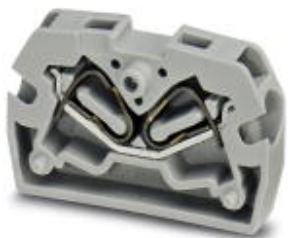
Mini flange terminal block, Connection method: Spring-cage connection, Cross section: 0.08 mm 2 - 4 mm 2 , AWG: 28 - 12, Width: 5.2 mm, Height: 22 mm, Color: blue, Mounting type: Screw mounting
