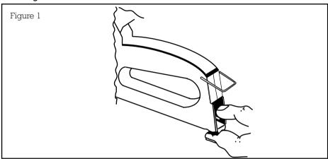
Squeeze and withdraw slide bar until stop is reached.
