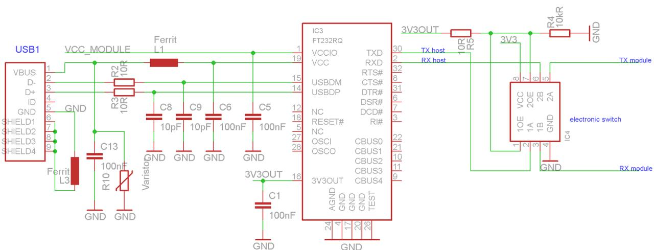
Figure 8: UART to USB converter: FT232R
