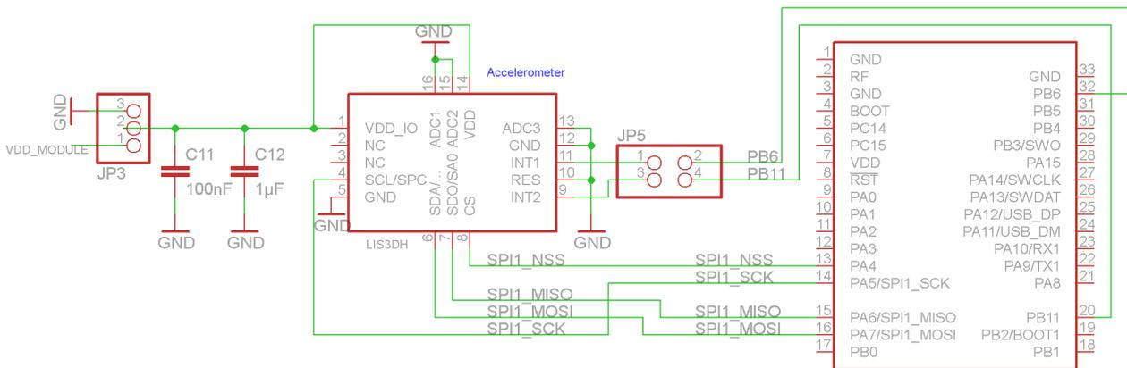
Figure 14: Connection of SPI accelerometer to module
